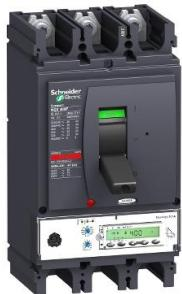
Circuit breaker, ComPact NSX400F, 36kA/415VAC, MicroLogic 5.3A trip unit 400A, 3 poles 3d
